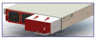
Using Handle, gently push By-Pass Module into the shelf
