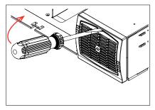
A) Use screwdriver to release the latch
