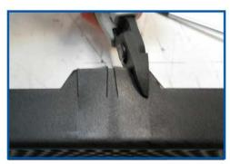
Cut holes to allow cable access
