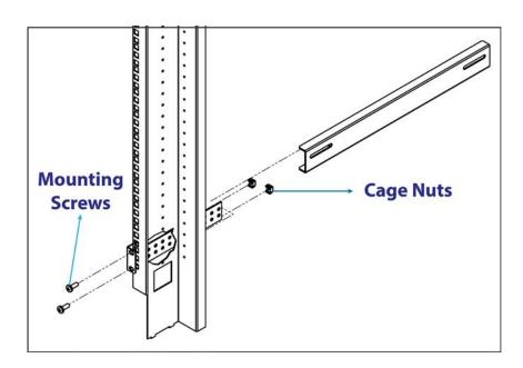
Assemble the sliders and adjust the length to suit the mounting depth
